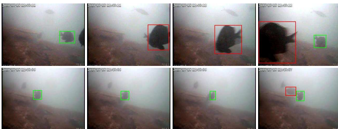
Figure 2: Fish-fish occlusions handled by the covariance particle filter. Let us note that the tracker is able to distinguish between fish with similar appearance and that move consistently in consecutive frames.
