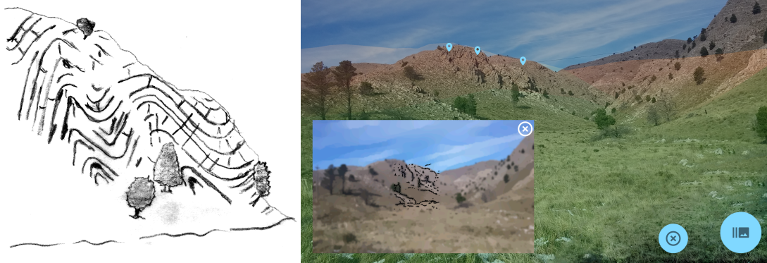
Figure 1: (Left) Common field sketch drawn by geologists during their usual workflow for analysis and interpretation of folded rocks. (Right) The proposed Augmented Reality (AR) system to assist geologists during the fieldwork. It allows the incorporation of geo-tagged information and it incorporates a sketch-like visualization (at the bottom left) that helps to analyze the complex geological structures.
