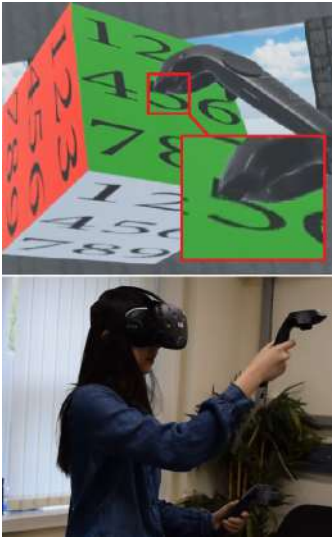
Figure 2: Users select their RubikBiom PIN by tapping with the dominant handheld controller on the cube that is attached to their non-dominant handheld controller.
