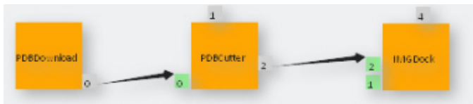
Figure 6: A gUSE workflow downloading a PDB file, splitting the stored complex into its receptor and ligand parts and performing a docking step.
