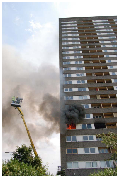
Figure 2. The BRE Center for Fire Safety Engineering at the University of Edinburgh and other partners in the FireGrid project conducted a series of large-scale fire tests in a high-rise building in Dalarnock, Glasgow. (figure courtesy of Rochan Upadhyay, FireGrid Project Team)
