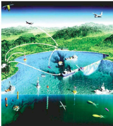
Figure 3: Observatory comprised of ships, aircraft and autonomous vehicles linked to assimilation modeling capabilities on shore
