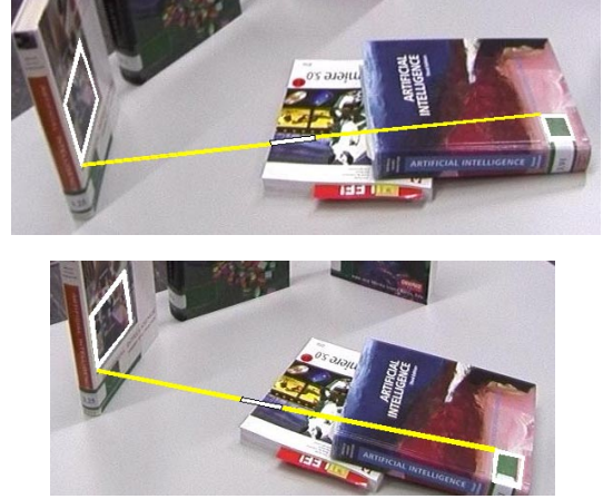
Figure 4: Top: Non-coplanar pair of regions. Bottom: Other view. The central line segment is misaligned.
