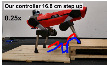
Figure 1.3: A snapshot of the robot walks on a flat surface, and climbs up a stair. The front leg trajectories are traced with red and blue lines. When the front legs hits and have been stopped, the algorithm infers there is a step ahead. Then, the agent comes up with a solution and has eventually climbed up the stair. (Image from the video)
