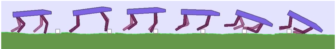
Figure 4.3: The baseline agent fails at a small stump (duration: 1s)
