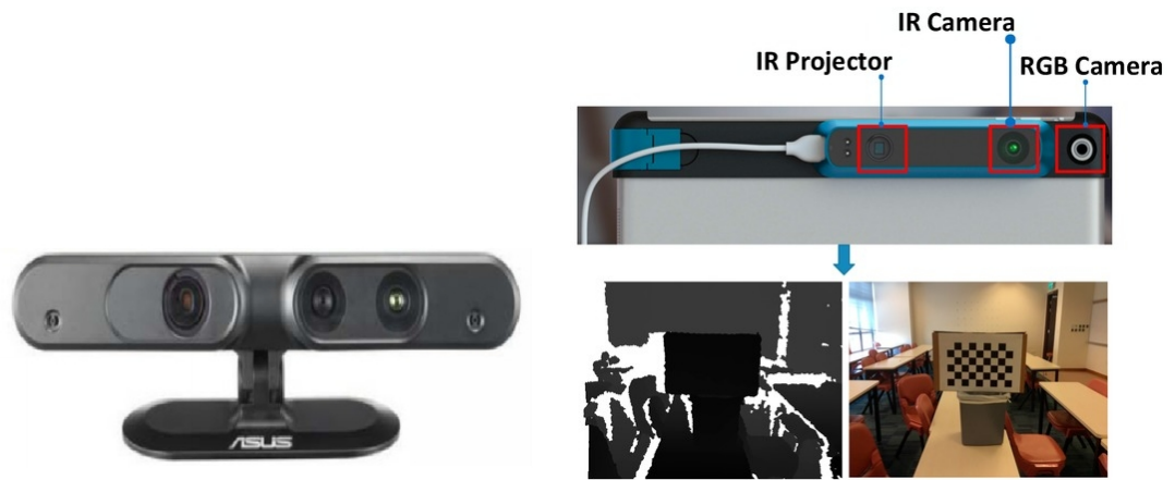
(a) Asus XionPro RGB-D sensor: Used for data collection.
